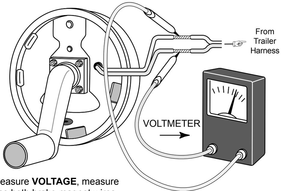
To measure **VOLTAGE**, measure across both brake magnet wires.
