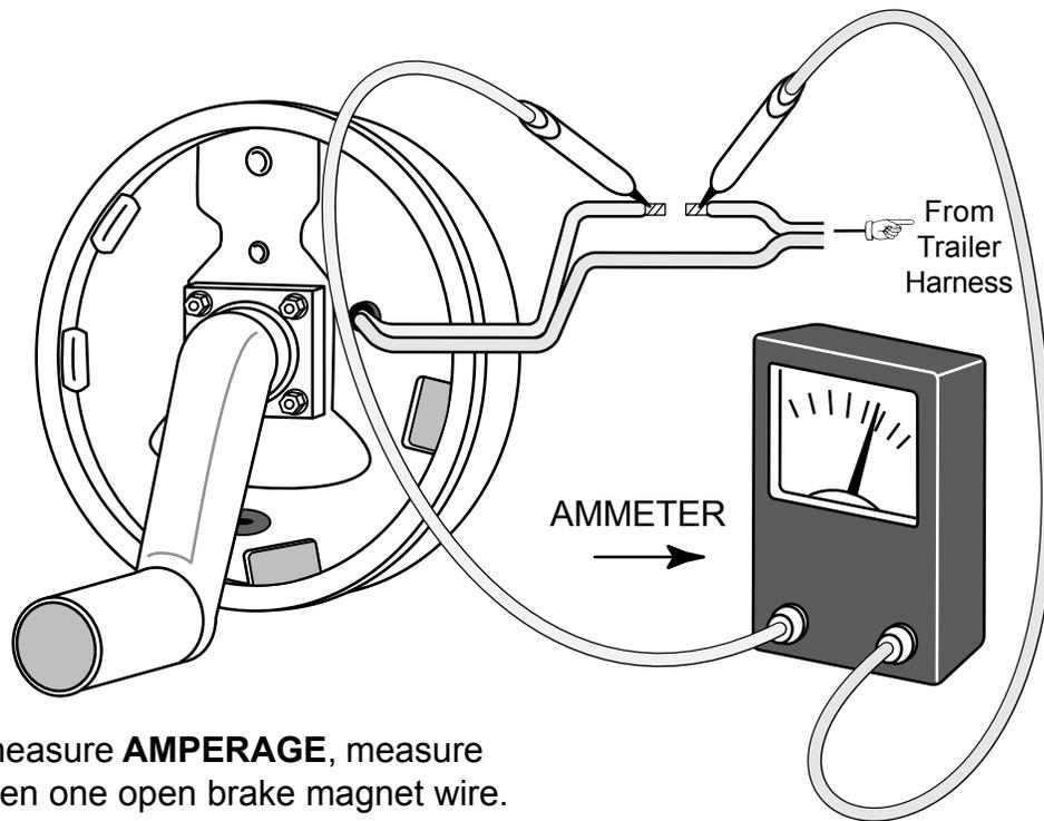
To measure **AMPERAGE**, measure between one open brake magnet wire.
