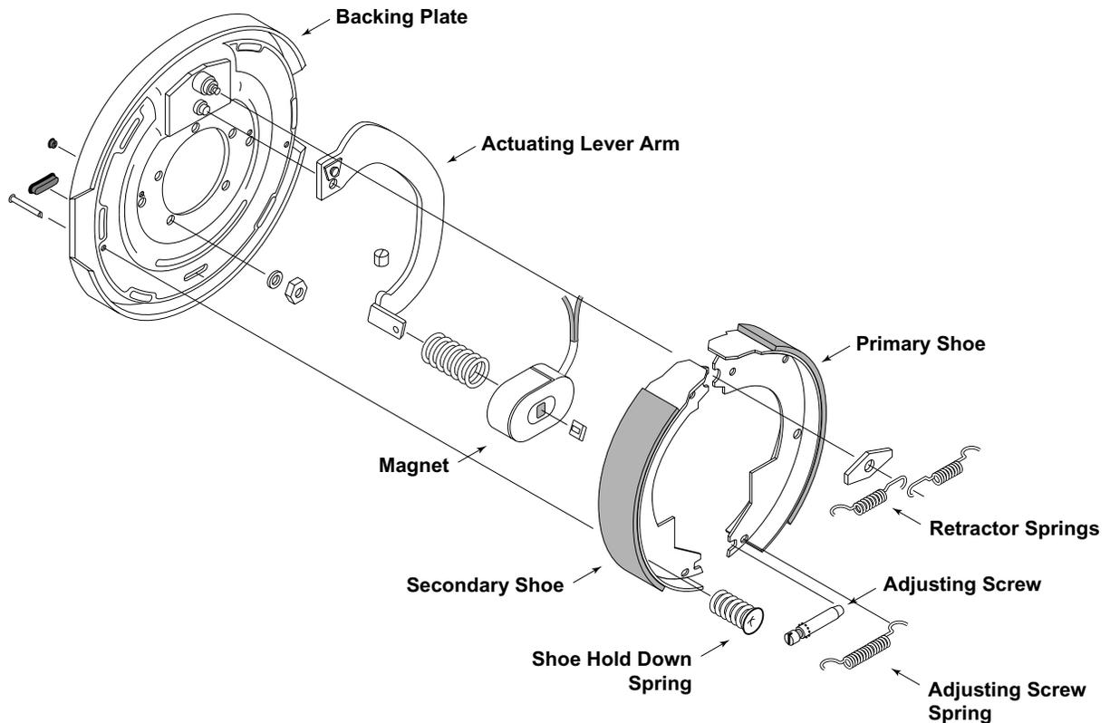
Increasing the current flow to the electromagnet causes the magnet to grip the armature surface of the brake drum more firmly. This results in increasing the pressure against the shoes and brake drums until the desired stop is accomplished.
