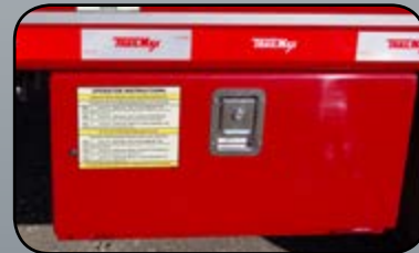
Self Contained 12 Volt Power Unit
