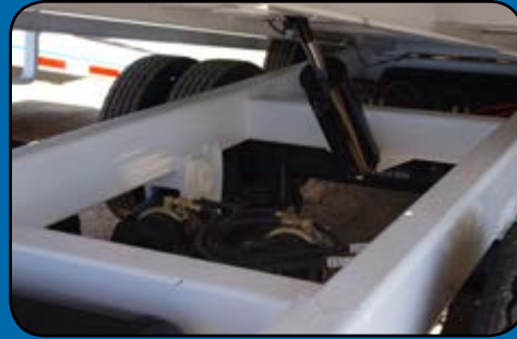
Cushion Cylinder for Load/Unload Control
