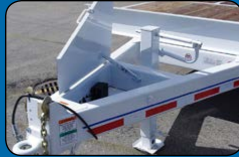
Lockable Storage Compartment in Tongue Area
