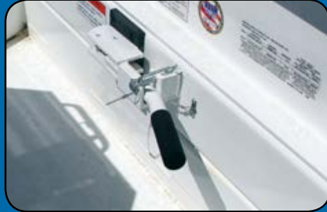
Over-Center Type Latch Assembly w/Tension Adjustment
