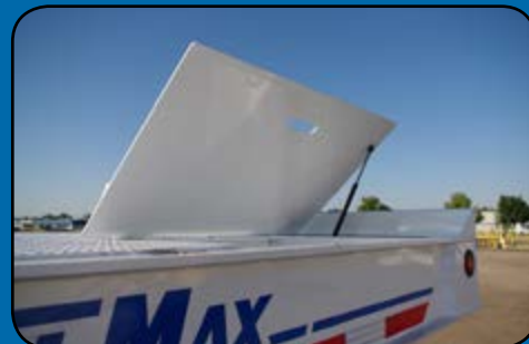
Storage Compartment in Upper Deck
