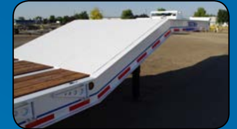
Riser Slope Angle of 20°
