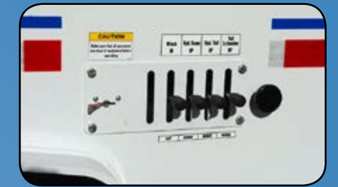
Hydraulic Controls at Gooseneck
