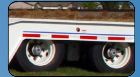
Air Ride Suspension with Dump Valve (on select models)
